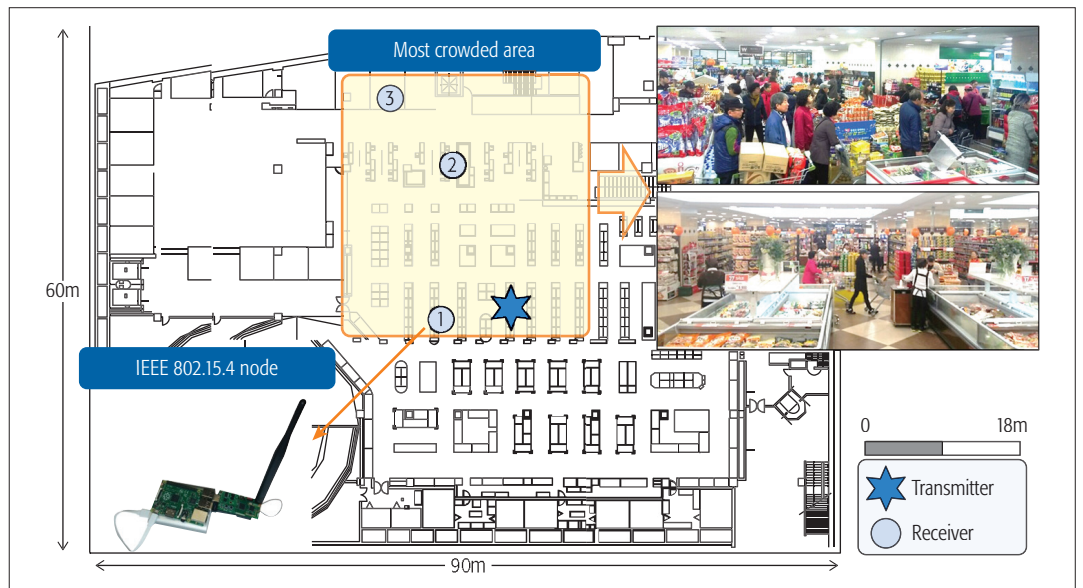
Figure 1. Link testing topology in a crowded urban market. We deployed a transmitter and three receivers in the most crowded area of the market for link quality testing.
