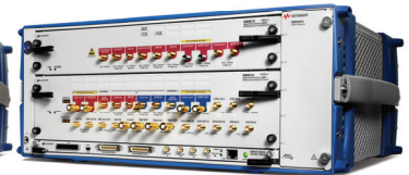
Keysight J-BERT M8020A high-performance BERT The most integrated solution for 100G Ethernet input testing
